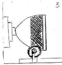
3. Presenting the tool at an angle will create small diagonal grooves. The method of changing the pattern of diagonal grooves can be achieved by presenting the tool at different
